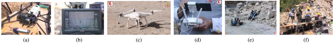
Fig. 3. (a) AscTec Falcon 8; (b) the video monitor of the Falcon's mobile ground station; (c) DJI Phantom 4; (d) customized remote control interface of the Phantom; (e) TRADR UGVs; (f) UGV base station; laptops provide interfaces for steering the robots and monitoring robot status and data acquisition.
